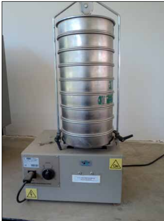
Figure 19: The electromechanical shaker with sieve plates.
