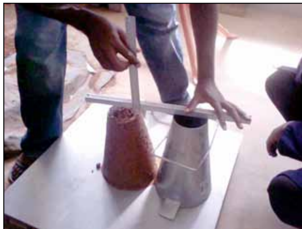
Figure 27: Measuring the slump of the fresh mortar. Source: Personal collection
