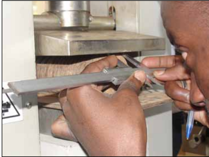
Figure 39: Recording the cross section area of the PETE bottle in contact with the platen
