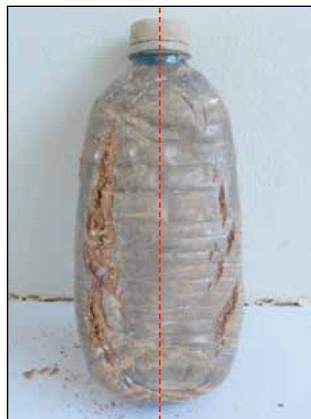
Figure 46: PETE bottle A4 at failure Source: Author
