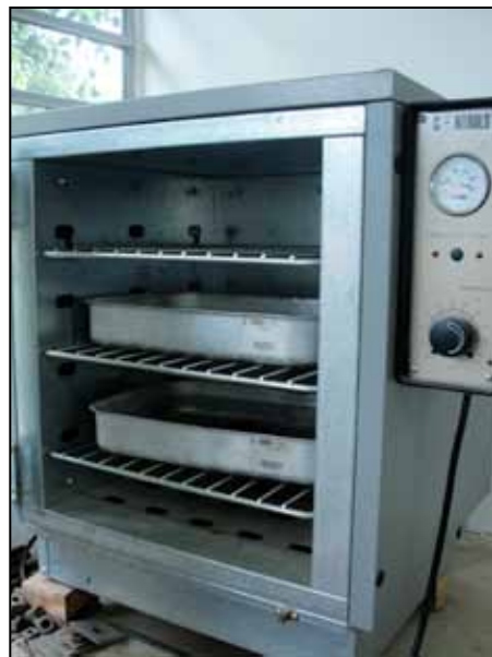
Figure 26: Soil specimen in the oven model CONTROL 10-D1390. Photo by author
