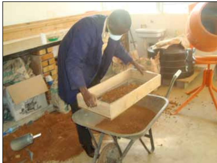
Figure 12: Sieving the soil specimen SM-UMU-A. Source: Personal collection
