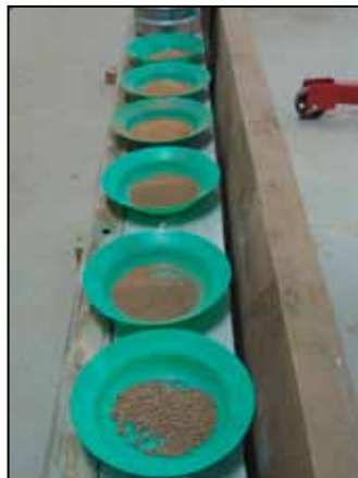
Figure 21: Sieved soil specimen on plates ready for weighing. Photo by authors
