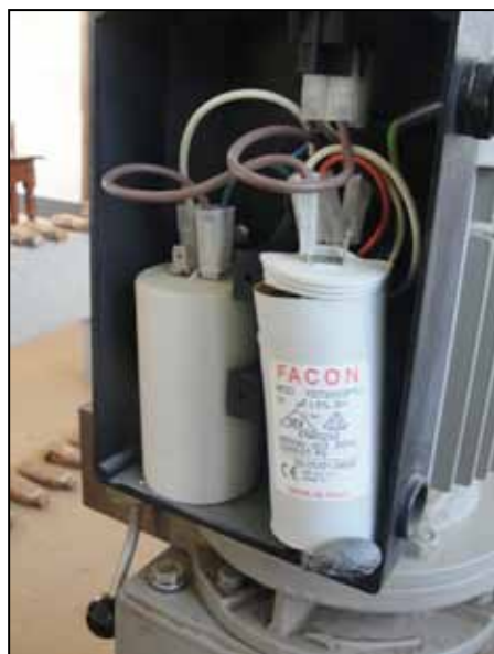
Figure 11: Capacitor that failed during test: Photo by Author
