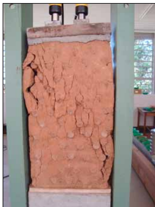
Figure 48: US-A-N1 Bond failure Source: Author
