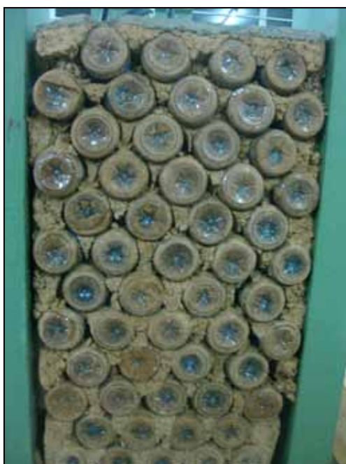
Figure 47: S-A-N1 Bond failure Source: Author
