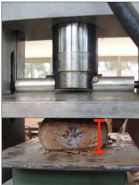
Figure 45: PETE bottle A4 unit under compression Source: Author
