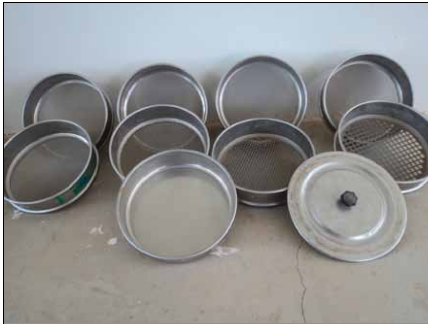
Figure 18: The sieve plates used for the dry sieving test. Photo by Author
