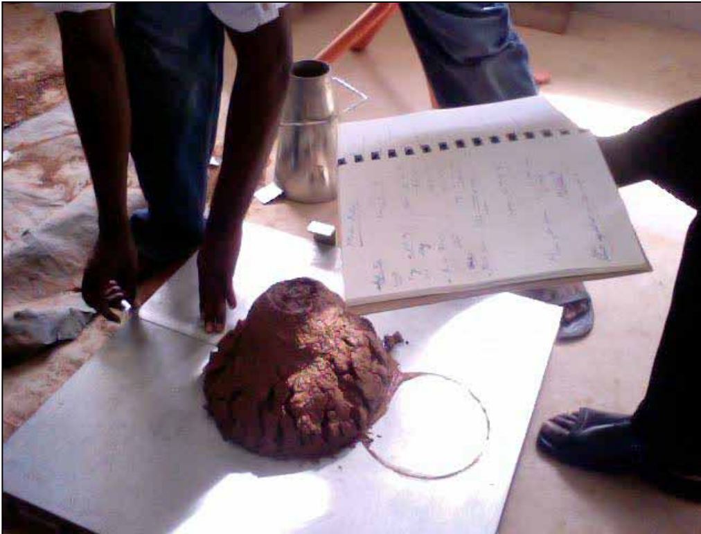
Figure 28: Measuring the flow of the fresh mortar. Source: Personal collection
