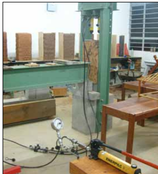
Figure 38: Hydraulic long ram jack machine installed on a modified steel frame support Photo by author
